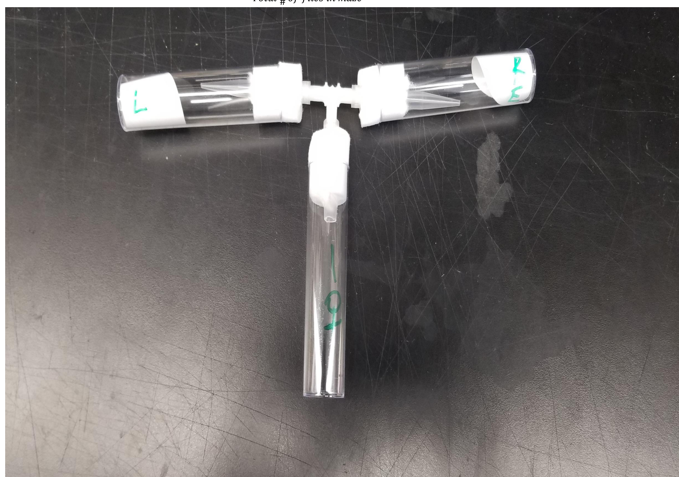
Figure 1: T-maze: The T-maze shown above is used to test for olfaction response to different concentrations of Apple Cider Vinegar (ACV). This behavioral assay utilizes pipette tips on each of its side to prevent the return of fruit flies back to the middle vial or out of the vial that was chosen first. Odors contained in the vial cannot escape into the environment, and as a result, the saturation is contained such that it is easily detectable by the fruit fly. The response rate and preference index can be calculated after the fruit fly has decided on which direction to follow.
