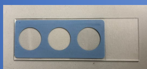
Image 3. Three well slides used in experiment. Cells are mixed with agar and then pipetted into each well before being irradiated.
