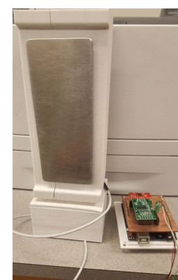
Figure 1: Grip/Load Force evaluation device for unimanual gripping [5]
