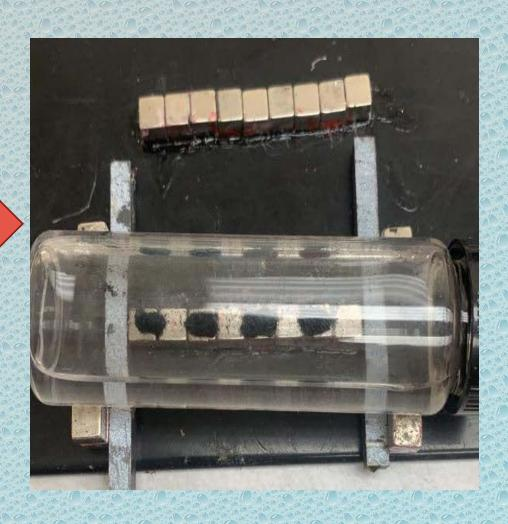
Figure 3. Halbach array of neodymium magnets aligned SWCNTs in fragmented depositions within a water solution due to reorientation along the greatest magnitude of magnetic flux generated across the magnets.
