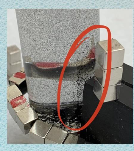
Figure 2. Secondary system designed with neodymium magnets to obtain alignment of SWCNT's within a medium through the reorientation of their magnetic dipoles.
